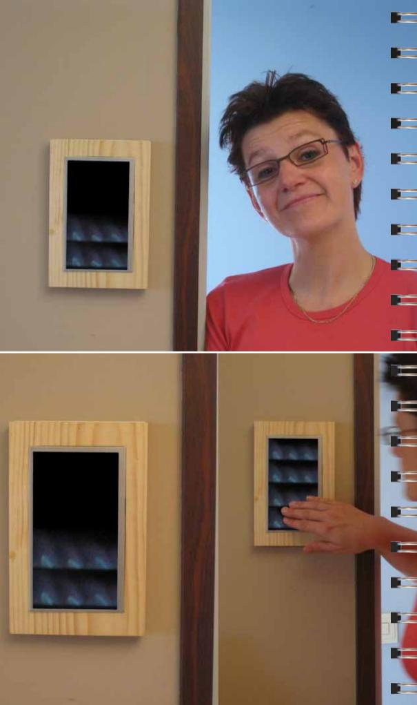
thermostat works like a very simple light switch and allows to change manually this programming: leaving a room for a while the user may set its temperature in stand-by mode, reducing energy consumption in consequence. When coming back with the intention to stay in the room for a sufficiently long moment, the user will switch off the stand-by mode and the room will get back to the 'presence temperature' set on the device.
